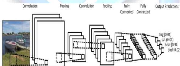
Figure 5. CNN Algorithm
